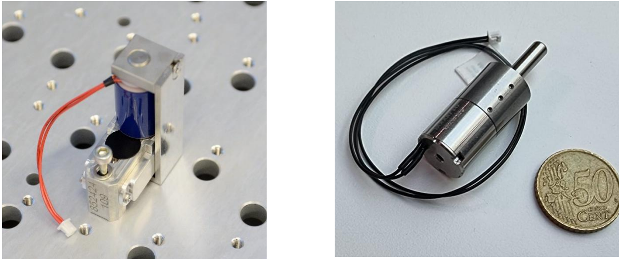
Figure 1-1: Hybrid Variable Reluctance (HVR) actuators developed by TNO, left shows the actuators developed for the UH2.2 ASM, and right shows the latest generation of actuators enabling an even higher force density and improved manufacturability.
